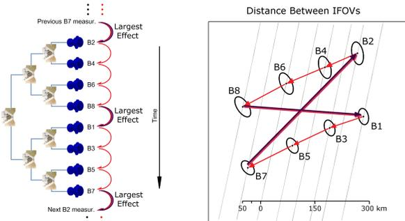
Evidence would indicate that each measurement is affected only by the preceding measurement. Analysis and tests show that this contribution between pairs of beams is always present between the same pair of beam and in all cases the mixing ratio of data is exactly the same. Results revealed a coupling percentage very close to 25%:
