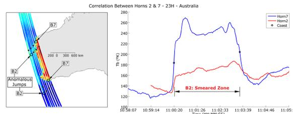
This figure above shows that beams 2 become warmer over ocean during the time beam 7 begin to observe land. Once beams 8 leave land the smear effect for beam 2 subside to expected scene temperatures. The effect is present in all beams but it can be seen that is more noticeable in beam 1 & 2. The next figures illustrate (in the right) the difference between the lines of sight of the MWR horns; in the left shows the sequence of contamination of the measurements.
