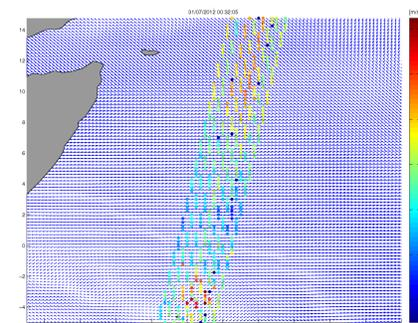
MWR wind speed and GFS wind direction corresponding to figures above.
