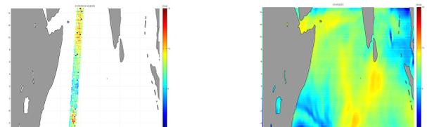
Extract of one pass for MWR wind speed at 00:32:05 31th July 2012 (left) and the corresponding GFS wind speed at the same time (right).
