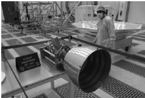
The Aquarius Ortho-Mode Transducer (OMT), around which the radiometer front-end components are mounted to achieve thermal stability. The Aquarius sunshade is also shown in the background. Photo was taken at JPL.
